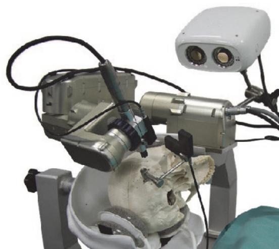
Fig. 1. Robotic system for minimally invasive cochlear access.
