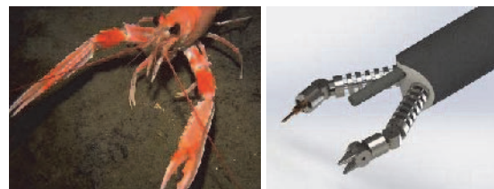
Fig. 1. Norway lobster (left) the CAD conceptual visualization of our proposed endoscopic robot (right)
