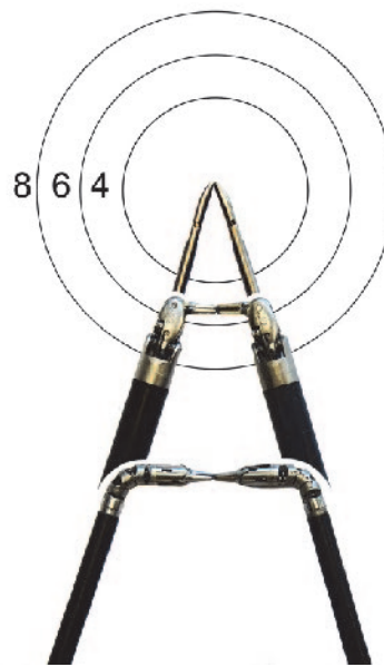
Fig. 1. Illustrative depiction of the 3 instrument pairs investigated (3mm non-robotic, 8mm robotic, and 5mm robotic positioned top, middle, and bottom respectively) in maximum positions of distal angulation. The 3 workspace diameter sizes (8cm, 6cm, and 4cm diameter) are infraposed and drawn to scale with respect to the instruments.
