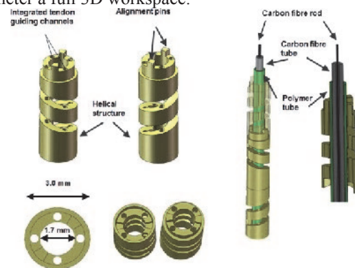
Fig. 1. Schematic view of the catheter design showing helical segments of the catheter (left) and through a cross-section (right)
