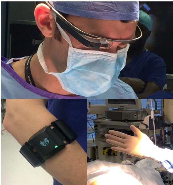
Fig. 1 (clockwise from top) First deployment of Google Glass for surgical guidance; Myo gesture control armband; open palm gesture used to engage orientation control.
