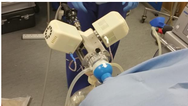
Fig. 3 In operating theater ready to operate on draped porcine patient. Shown are airtight port, tool mounting rails, actuation pack, and endoscope. Insufflation attachment at sides.
