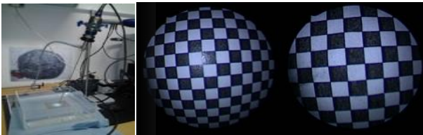
Fig. 1 Images of a calibration target acquired with a fetoscope. Left: calibration setup. Right: images of the calibration target respectively in the air and in water.
