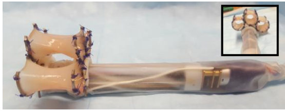
Fig. 2 – Ex vivo test on sheep bowel. Three segments of small intestine are sutured to the rings with six sutures each.
