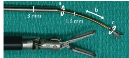
Fig. 1 Tube configuration: Outer Tube - straight, steel fixed to tool base. Middle Tube - curved, nitinol with rotation (a) and translation (b). Inner Tube - straight, nitinol with rotation (c). Included is an 8mm instrument for size comparison.
