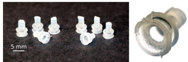
Fig. 2. Left, fabricated prototypes of suction based soft grippers, right, zoomed view of the gripper.
