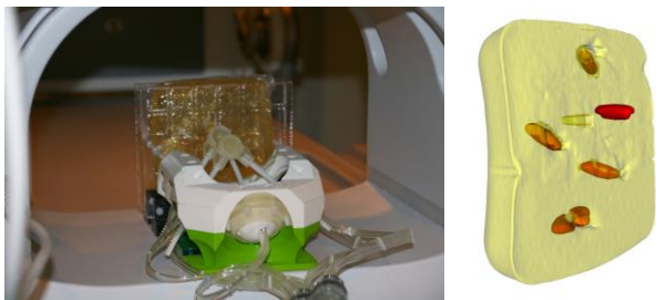
Fig. 4 Left: Measurement setup in a 0.25T MRI scanner. Right: 3d rendering of the ex vivo tissue phantom, made out of gelatin (yellow) containing four fish oil capsules (red). The fifth marker is attached to the needle.
