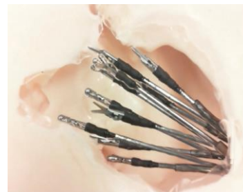
Fig. 3 Intraventricular reachability evaluation in a silicon brain phantom.
