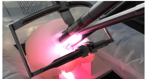
Fig. 1: da Vinci® Xi with 8 mm instruments performing a cleft palate repair on the cleft palate phantom.
