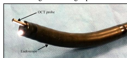
Fig. 2 OCT probe inside the endoscope.
