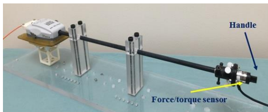
Fig. 3 Experimental setup for evaluating the performance of force sensing.
