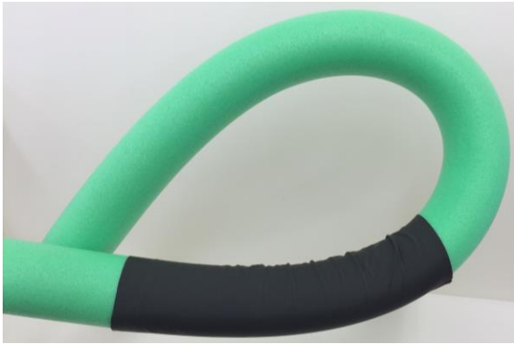
Fig. 2 Experimental deformable body. A foam cylinder (green) is used to have the shape of a medical tool. EIT measures are taken over a highly conductive textile (black) that is placed over the cylinder.
