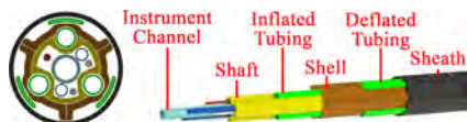
Fig. 3: A section view of the main body. All components that lie along the main body can be seen. Instrumentation channel, CO 2 /water channels, lighting fibers and camera cabling are at the center of the shaft. Inflated tubings lie between the shaft and shell while deflated tubings slide between the shell and sheath.
