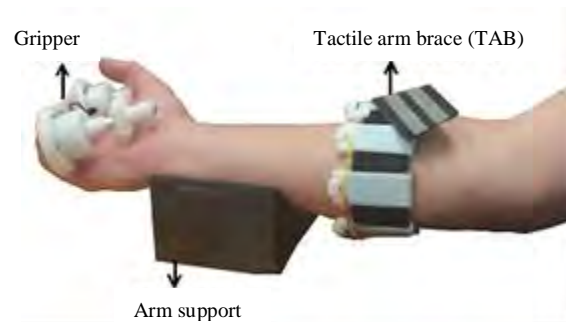
Figure 1 Participant performing gripping motions with the gripping device while wearing the TAB (tactile arm brace).
