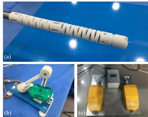
Fig. 1 System components of K-FLEX. (a) The overtube has four degrees of freedom (DOF), one translation movement and three rotation movements(roll, pitch, yaw). (b) The master device has the same kinematic structure with overtube except grasping. (c) Foot clutch is used to extend the master device's working space.
