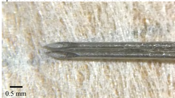
Fig. 4 Image showing the layout of the two 30 gauge needles glued side-by-side with the injection needle (bottom), slightly leading the needle carrying the OCT fiber (top).
