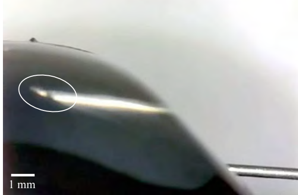
Fig. 3 Deformation of the endothelial layer as the needle pushes against it before penetrating into the anterior chamber. Test performed with 25 gauge needle in fresh cow eye at 75°.
