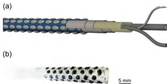
Fig. 1 Tubular pressure-sensitive soft sensor skin. (a) Illustration of a concentric tube soft robotic arm covered with a pressure sensor array. (b) Prototype sensor with 8×8 tactile pixel array and wire electrodes embedded in a soft silicone rubber carrier membrane; the outer diameter is 7 mm.
