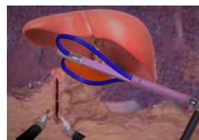
Fig. 1: Concept of the organ retraction (or liver retraction) using proposed retractor. The retractor beam (blue one) was expanded to support the liver.
