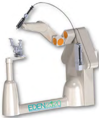
Fig. 1: EDEN200 robotic system render: the robotic catheter driver is integrated within the hardware of the neuromate ® (Renishaw Plc)
