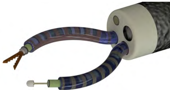
Figure 1: Conceptual drawing of a dual-channel flexible endoscope with our luminal manipulators delivered through its ports.
