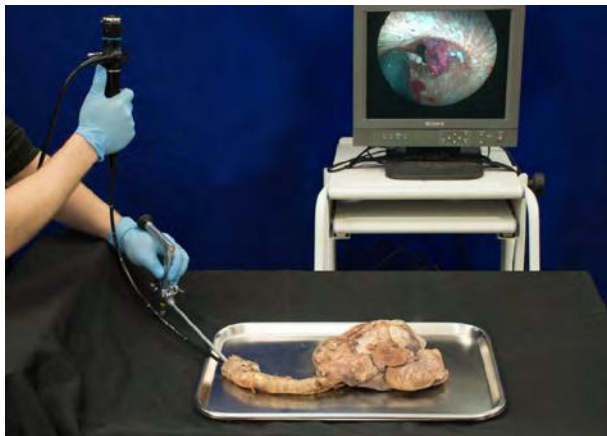
Figure 4: Experimental Setup: The bronchoscope was used to deploy the luminal manipulator into the sheep trachea. A rigid endoscope was introduced beside it to capture the images shown in Figure 3.
