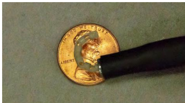
Figure 2: Prototype luminal manipulator delivered through a 6 mm diameter bronchoscope.
