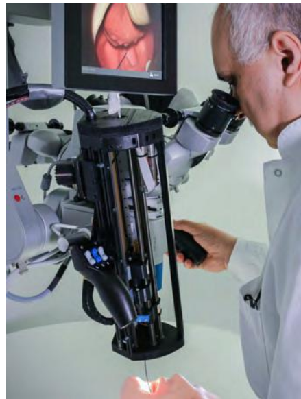
Fig. 1: Example of an integrated setup with a concentric tube robot and a surgical microscope.
