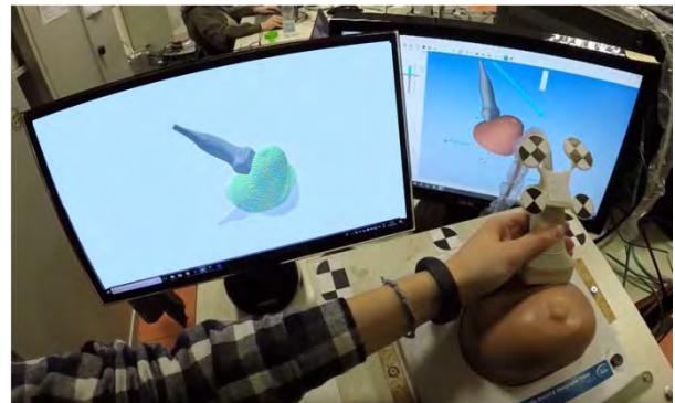
Fig 1. The FUS system allows to map the real positions of the CIRS breast phantom and the US probe to the 3D Slicer scene (right monitor). Information about probe spatial transformation is communicated to the simulated environment in Unity (left monitor).
