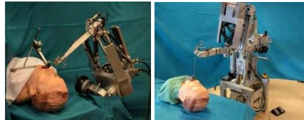
Fig. 1, 2 Standalone REMS (left) and REMS + PPS (right)
