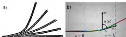
Fig. 3 a) Configurations of the distal SRMC segment q values. b) Parametrization of continuum segment shape.
