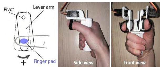
Figure 3. Scheme for one actuator of the haptic device (working principle) and views of the entire device.
