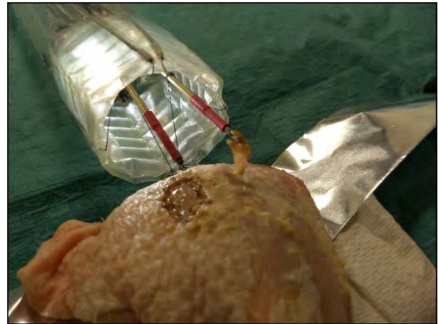
Fig. 2: The inflatable robot having removed a section of skin from ex-vivo chicken breast tissue.
