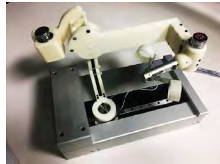
Fig. 4. Assembly of proposed master device featured redundant joint for 4-DOFs slave of flexible surgery robot.
