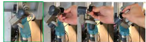
(a) Well chosen initial configuration allows smooth orientation movement in the subsequent tele-operation
