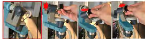
(b) Badly chosen initial configuration results in frequently hitting on the joint limit
