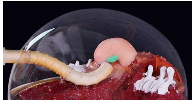
Fig. 1 Concept and application scenario of the endoport system in an in vitro human abdomen. A potential renal tumour location is marked in green on a silicone kidney.
