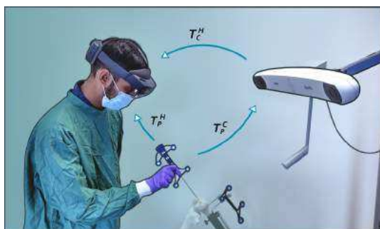
Fig. 1 A co-registered AR surgical workflow, using the HoloLens 2 and Navio ® system. T_C^H : calibration matrix between tool pose in virtual world-frame T_P^H and surgical coordinates T_P^C .
