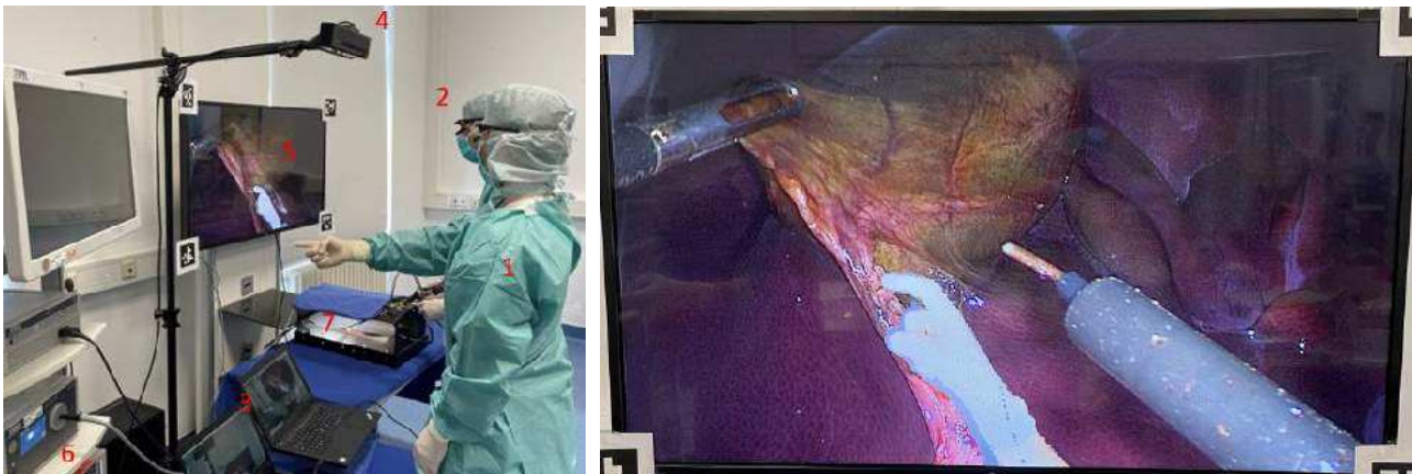
Fig. 1 Left: Instructor (1) and trainee (2) wear Pupil Core eye-tracking glasses connected to separate laptops (3). When using the iSurgeon the instructor (1) works with hand gestures detected by a sensor (4) to instruct the participant (2). The gestures are projected on a screen (5) connected to a laparoscopic tower (6). Tasks are performed in a box trainer (7). Right: The expert's hand is displayed on the laparoscopic screen while he instructs the trainee to perform a porcine laparoscopic cholecystectomy (task 8).
