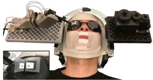
Fig. 1 Radiotherapy immobilization system modified to enable surgical robots to be quick-connected magnetically through a standard surgical draping (not shown). System shown fitted with one robot and counterweights for balance. (Inset) In this study, tracking markers placed on the robot and goggles are used to quantify the displacement of the robot relative to the goggles (i.e., the eye) due to breathing/snoring motion of the wearer.
