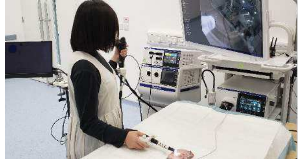
Fig. 3 Ex-vivo test setup: a commercial endoscope system, and the diathermy machine; the passive bending overtube and the translation actuation module were installed on the endoscope to channel the robotic lifter; a cart for actuation motors is located beside the operator who held the controllers of the endoscope and the robotic lifter in separate hands.
