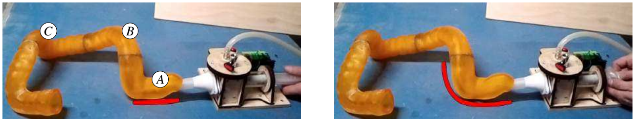
Fig. 2 The experimental setup. The EndoVine travels through the rectum (A) into the sigmoid curve (B). It adapts its shape to overcome the curve to reach the splenic flexure (C).
