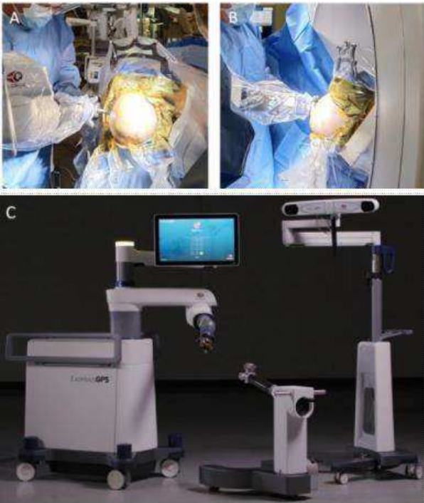
Fig 2. Surgeon guides the robotic arm (A and B) for sEEG depth electrode placement. ExcelsiusGPS robot (C. From left to right: Robot system with real-time display and robotic arm with end effector attached, patient stabilization device used in cranial procedures, camera system).
