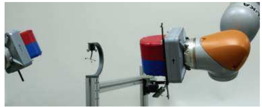
Fig. 1 Experimental set up: a manipulator with optical markers, robotic arms with External Permanent Magnets (EPMs) and frame with optical markers.
