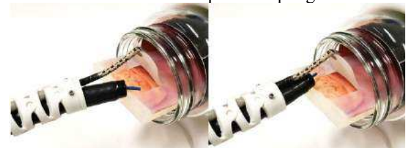
Fig. 2 A silicon rubber mimicked mucosa tissue is used to demonstrate an RTD-assisted endoscopic resection, both the lifter and the dissector can be controlled independently, and their motions are decoupled.
