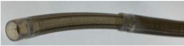
Fig. 1. Example tendon-actuated catheter comprised of two telescoping tubes.
